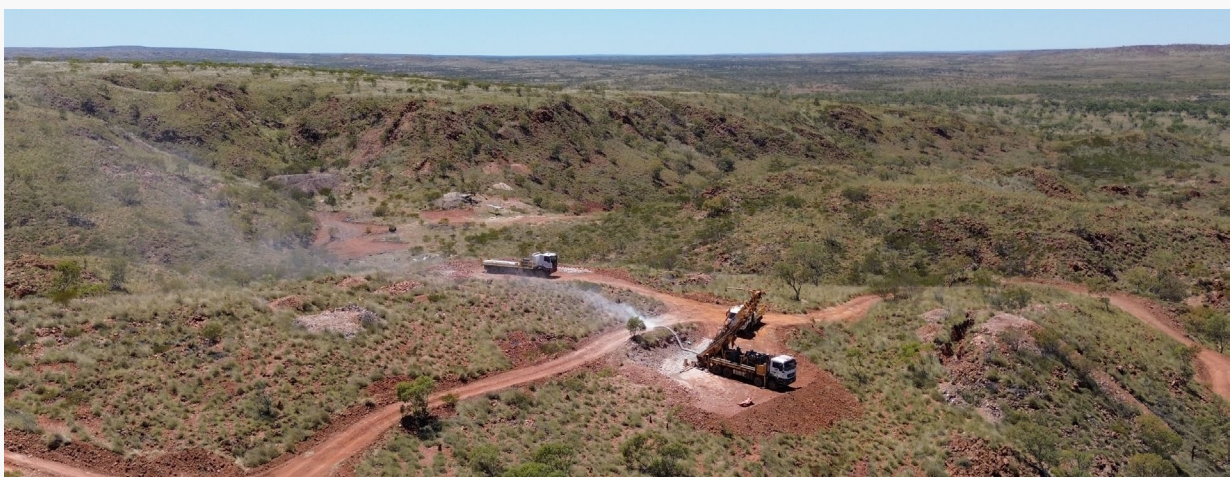
Figure 8: RC drilling at the Bonanza with Black Diamond working in the background.
